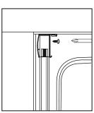
6 - Whilst ensuring that the bottom of the assembly is held snug to the shower tray and that all parts are level and upright, fix the assembly to the wall channels by drilling through the pre drilled holes in the wall channels into the profiles of the fixed panels using a 2.75 mm metal drill bit. Then secure using 6 x ST3.5x10 short screws (4 per wall channel).
