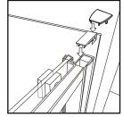
10 - Once you are happy that the installation is correct and that the doors are running smoothly, push the cover caps onto the top of the wall channels as shown, (smaller top cap first followed by the larger wall channel top cap).
