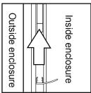
7 - Push the shorter 2 of the 4 water seals onto the exposed glass edges of the fixed panels, the flaps should face into the shower as illustrated.
