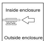
8 - Attach the handle making sure that the rubber washers that come with the handle are placed between the handles and the glass.
