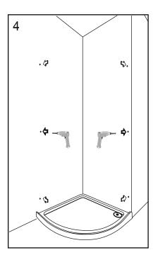
4 - Remove the assembly and drill the marked points using an 6 mm masonry drill bit, once this is done insert 8 x wall plugs into the holes.
