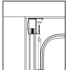
5 - Reposition the assembly and fix the wall channels to the wall using 8 x ST4x30 long screws (4 per channel)
